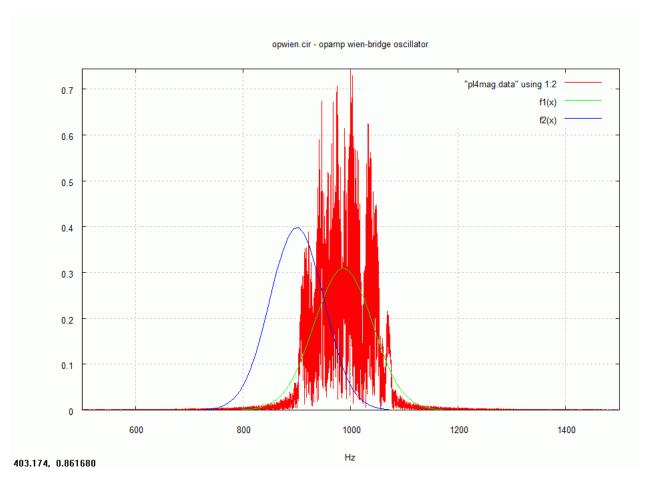
pl4mag.data is the simulation data, f2(x) the starting curve, f1(x) the fitted Gaussian distribution. This is just a simple example. You might explore the powerful built-in functions of Gnuplot to do a much more sophisticated statistical data analysis.
