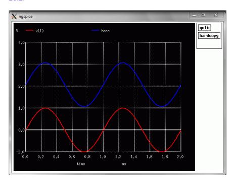
Figure 21.2: node 1 and node 'base' versus time
