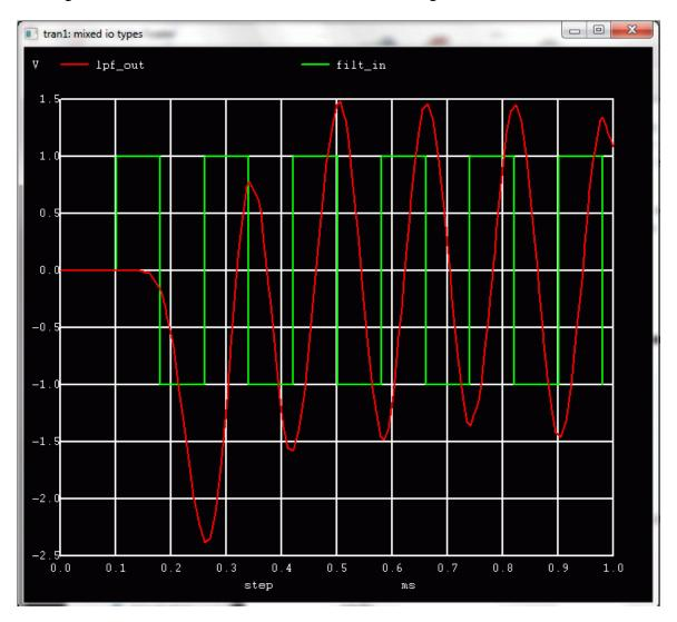
Figure 27.3: Nutmeg Plot of Subcircuit Internal Node
