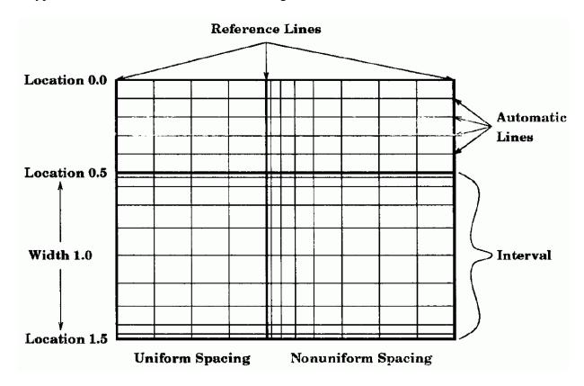
Figure 30.3: Typical mesh for 2D devices
