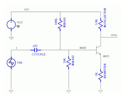
Figure 21.1: Transistor Amplifier Simulation Example
