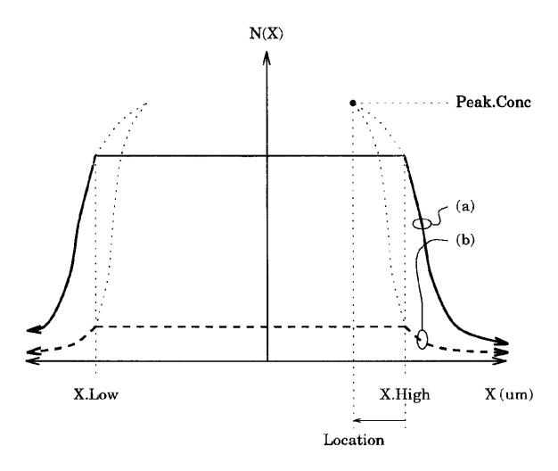
Figure 30.2: 1D doping profiles with location < 0.
