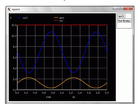
Figure 21.3: VCC, Collector and Emitter Voltages
