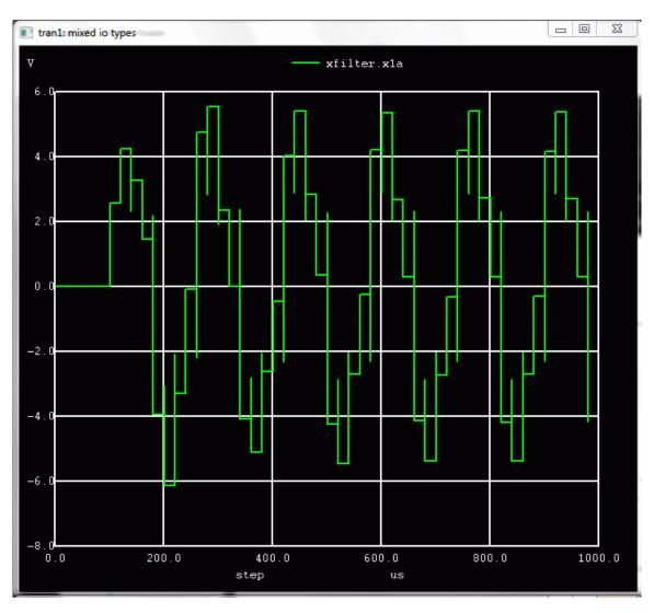
Figure 27.2: Nutmeg Plot of Filter Input and Output
